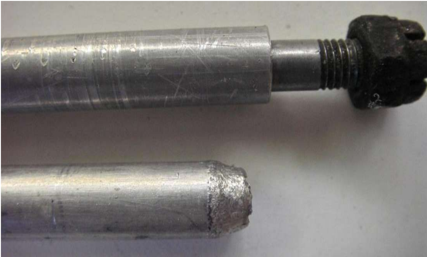
Photo 3 Rear hanger thru-stud, showing worn starboard end of under-length alloy spacer (compare with new full-length spacer at top)
