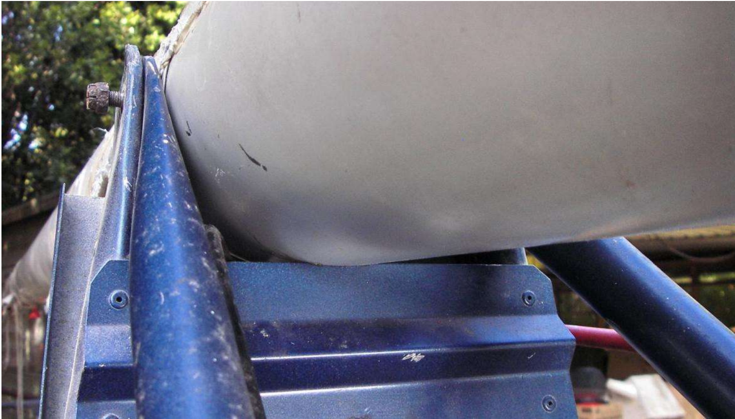
Photo 1 View of rear hanger attachment, with boom resting on alloy gusset.
